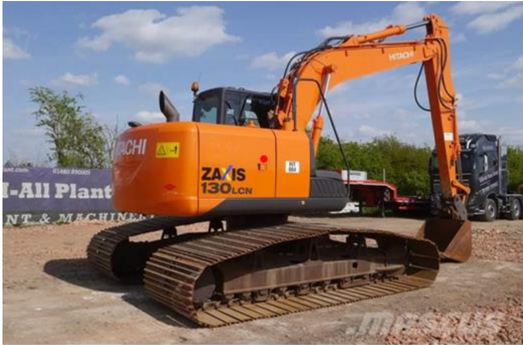
Plate 2-1: Wide-Track Excavator (Bog Master)
